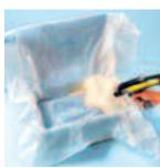
3 The lid is closed. The foam expands inside the pre-mold box. A few seconds later the foam has set.
