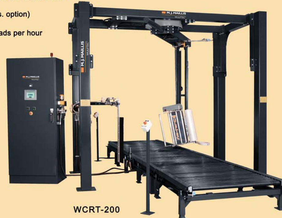
WCRT-200 SELF-SUPPORTING 4-LEGGED MODEL
